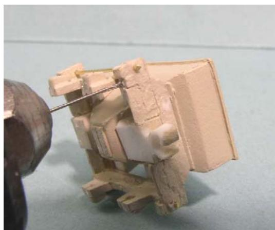
20. (left) Drill the end sills .012 (#80) for the brass wire journal reinforcement bars.
