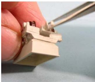
6. If you're using the dummy knuckle coupler, trim flash out with a sharp #2 blade, and check fit with your normal coupler. Make sure there is sufficient 'slop' for some twist and vertical movement. When satisfied, glue the coupler box in the frame end pocket as shown. The 'link and pin' box mounts in the same manner if you use that option.
