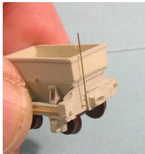
17. Drill the various hole locations .012 (#80) with a pin vise or a Dremel on low speed. Bend a piece of .010 wire and ACC in place for the vertical brakeshaft. Don't worry on length, it can be trimmed back later. If you want, fashion a tiny "U" from wire and make a top bracket to secure the handbrake shaft to the top edge of the hopper; drill and ACC in place.
