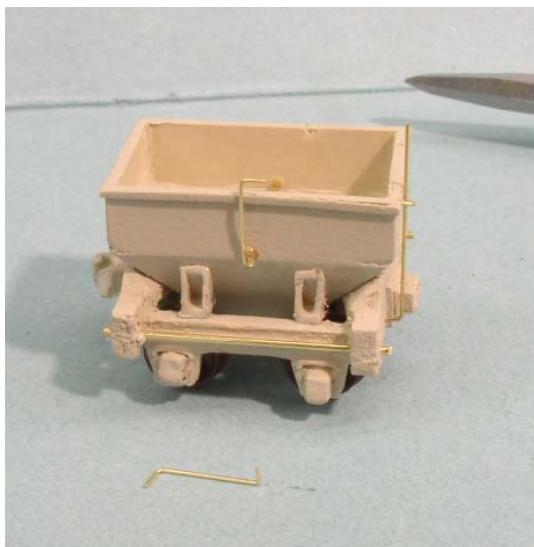
18. (left) Bend a piece of .010 wire for the unloading crank as shown. ACC in place on the side. The “crank” handle seemed to be normally positioned parallel to the car side edge.
