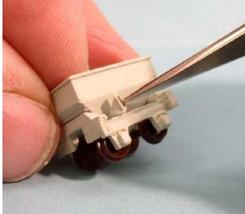
2. Remove remaining edges and flash across the top of the 'hopper' casting. Run a flat mill file across the top to flatten and smooth the top surface. Prototype thickness was 1x2 angle iron on the top edge.
