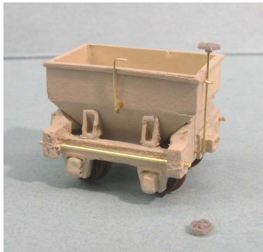
22. Trim the top of the handbrake shaft to desired length and ACC the brake wheel on top. Photos show brakemen standing on the ore loads with the brakewheel at waist level, so use that as a general height guide.
