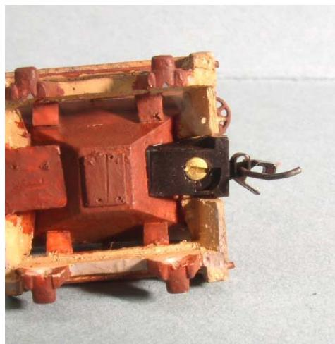
7. Z coupler boxes can be installed by cutting a hole in the hopper body frame as shown with a sharp #2 blade. Remove wheels. Score lightly and cut intentionally small, then trim opening to fit the back of the coupler box. Drill frame .035 as shown for a 00-90 screw; tapping not necessary. Also note how the coupler trip pin is rebent.
