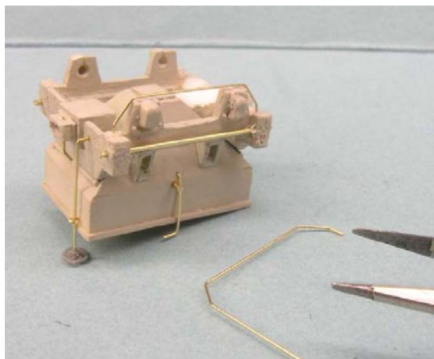
21. Bend .010 wire to the shape shown at left, and fit into the sill holes and across the bottom of the wheel journal boxes. Take your time on this step. ACC in place.
