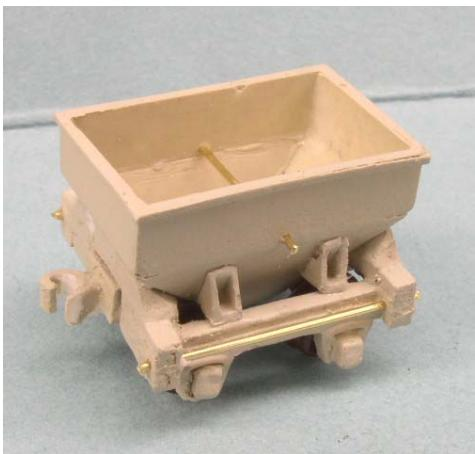
14. ACC the .020 rods in place. A needle works best to transfer small amounts of ACC to the carbody, rather than use the tube nozzle. Also keep a little tissue handy to blot/wick out excess ACC if it does happen.
