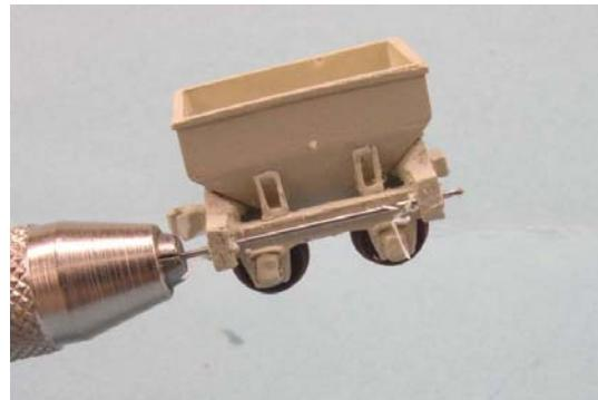
13. Insert and trim .020 brass wire for the unload crank shaft (left) and the side reinforcement bars (below)
