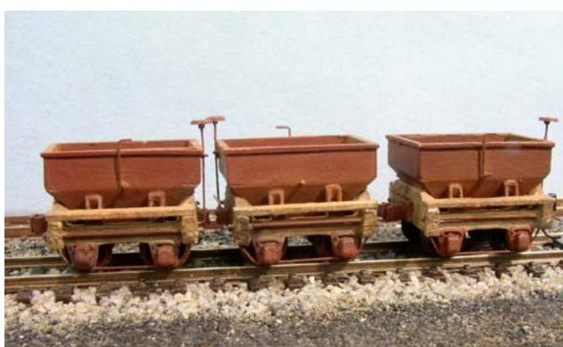
28. I used AIM weathering powders for the final finishing; medium earth for the hopper bodies and wood and a little black for the details.
